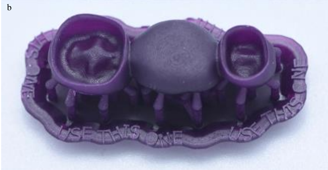
Figure 2. Additive Manufacture Patterns: Intaglio surface of patterns fabricated by additive manufacturing -- (a) Castable Resin, (b) Castable Wax. Sprues were not removed due to only analyzing intaglio surface.
