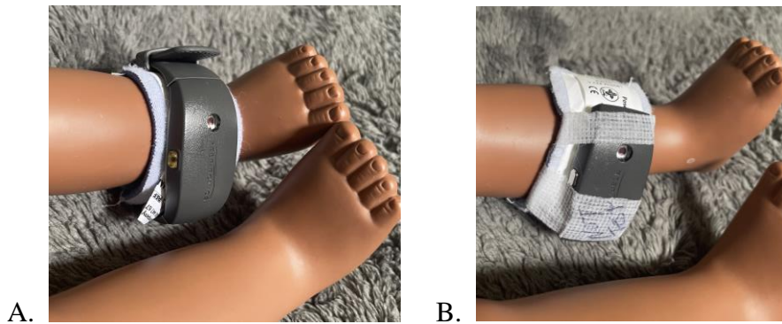
Figure 2. Picture of actigraph used for study. A. Actigraph with straps on placed over top of soft band. B. Actigraph taped to soft band.
