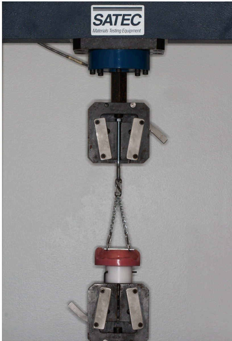
Figure 5 Application of tensile force using a universal testing machine.
