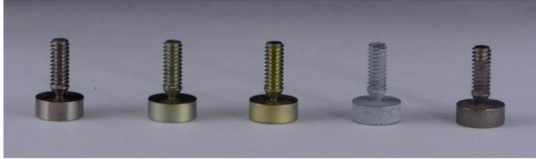
**Figure 1 Five different surface treated miniature implant specimens from left to right: (1) Machined 0.3 - 0.4  $\mu\text{m}$ ; (2) Anodized 0.3-0.5  $\mu\text{m}$ ; (3) Anodized 0.8  $\mu\text{m}$ ; (4) SLA 1.6  $\mu\text{m}$ ; and (5) BST 1.0  $\mu\text{m}$**
