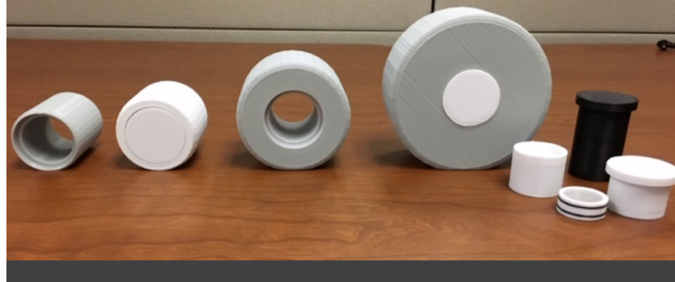
Various cylindrical phantoms designed by Dr. Polf using Tinkercad.com, and printed at the HS/HSL Innovation Space. Photo by Jeremy Polf.
