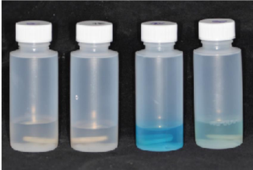
**Figure 4:** Samples soaking in distilled water, 6% alcohol, Prevident, and chlorhexidine, respectively.
