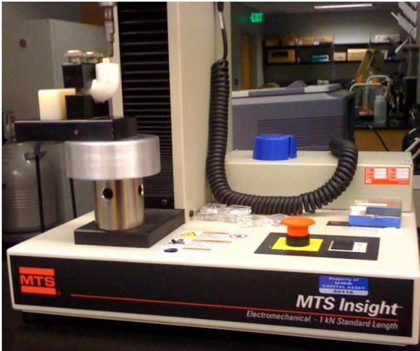
Figure 4 – Tooth sample in place prior to testing. Shearing blade was used to break the enamel/adhesive bond.
