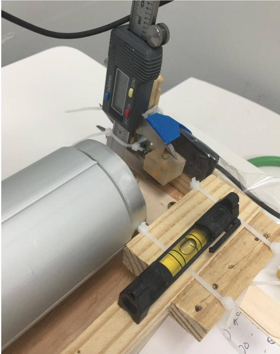
Figure 1: Radiographic Sensor Alignment and Crown Measurement Jig
