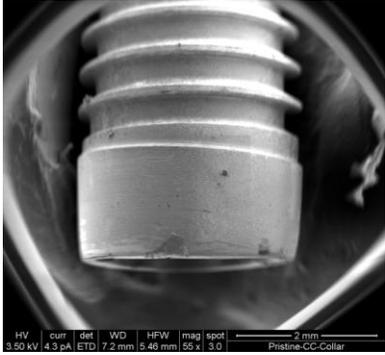
Figure 20: Calcium carbonate at 50x demonstrates several gouges
