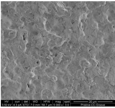
Figure 24: Calcium carbonate causing extensive obliteration of pores at 5000x
