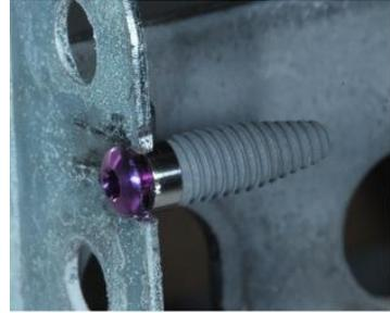
Figure 3: Implant mounted on onto jig with notch facing out
