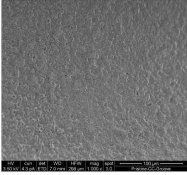
Figure 23: Calcium carbonate at 1000x shows minimal identifiable pores present
