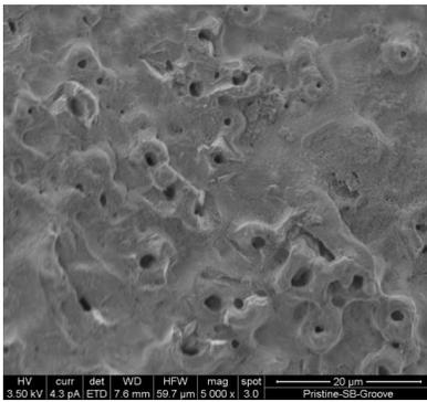
Figure 15: Sodium bicarbonate at 5000x. Partial and full obliteration
