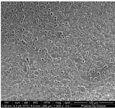
Figure 18: Glycine exposure at 1000x, and minimal changes noted vs. control
