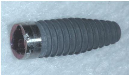
Figure 12: Visualization of sodium bicarbonate surface coating
