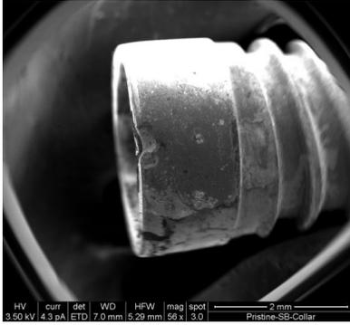
Figure 11: Sodium bicarbonate exposure at 50x. Notch and surface coating noted
