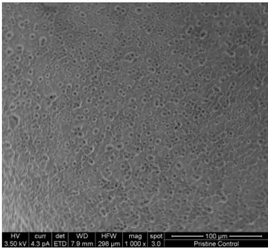
Figure 9: Control at 1000x used for analysis. Micro-porosities clearly
