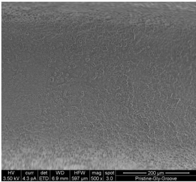
Figure 17: Glycine exposure at 500x. Note the groove is centered within the threads
