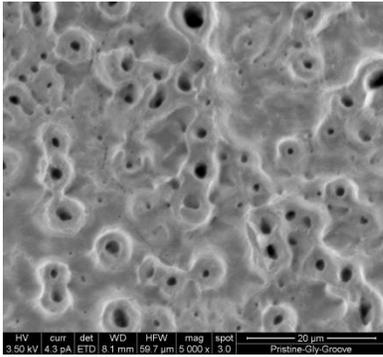
Figure 19: Glycine exposure at 5000x shows similar complete and partial pores with border
