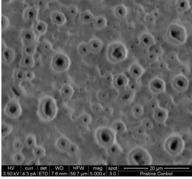
Figure 10: Control at 5000x. Irregular geometry and nano-porosities
