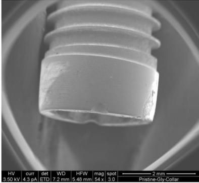
Figure 16: Glycine at 50x magnification showing notch and lack of surface coating
