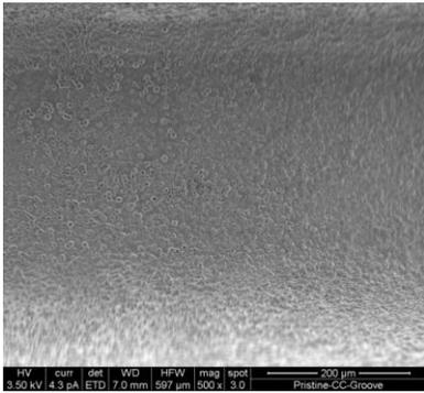
Figure 21: Calcium carbonate at further magnification at 500x shows absence of pores
