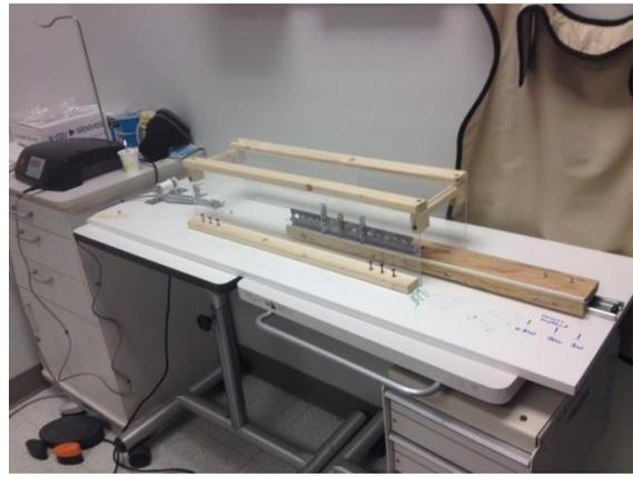
Figure 5: Complete view of implant mount, track, plexi-glass enclosure, and implant motor
