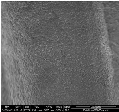
Figure 13: Sodium bicarbonate exposure at 500x. Note the groove centered within threads
