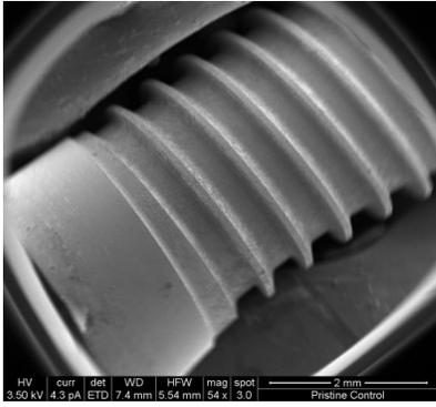
Figure 7: Control implant at 50x. Note reference notch, threads, and
