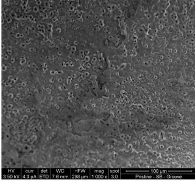
Figure 14: Sodium bicarbonate at 1000x. Devoid and altered areas
