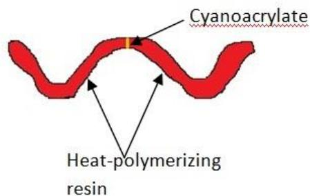
The fractured denture and the cast were matched together according to the number labeled during the preparation. The repaired denture base was allowed to set for five minutes before removal from the master cast for polishing. A photograph of the denture base repaired with Loctite Superglue Professional is shown in Figure 5.
