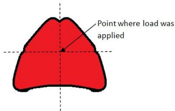
The first line connected the buccal frenum notches on the left and right; the second line was perpendicular to the first line and drawn from the labial frenum notch. The intersection of these lines was the location where the load was applied.
