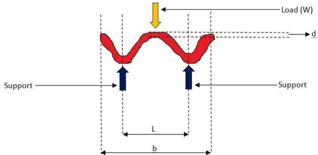
The transverse fracture strength,  $S$  (Pa) of each specimen, was determined using the following formula:
