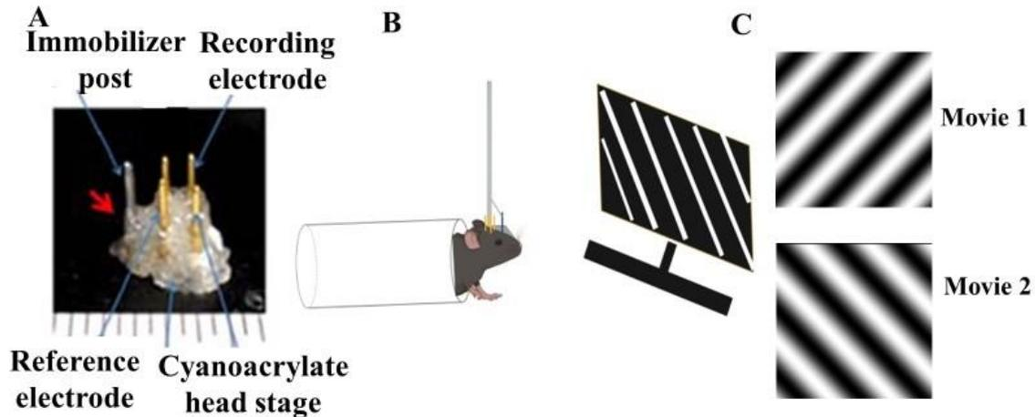
**Figure 4: Head stage and VEP setup.**
