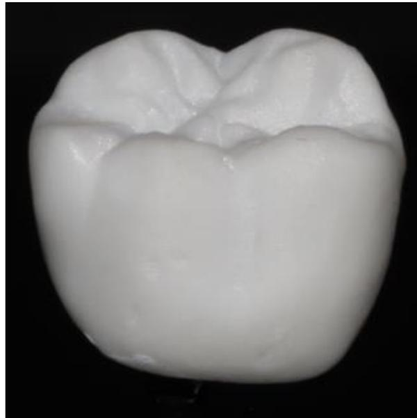
**Figure 2.** Additive manufacturing specimen. Specimens were produced by digital light processing (DLP) using the Ember printer from Autodesk. Printed specimens were subject to post-production sintering and polished using the 2-step zirconia polishing kit by Brasseler.
