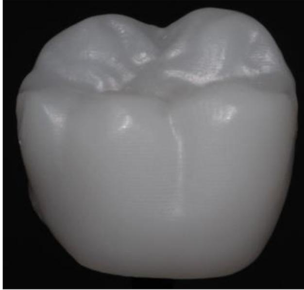
**Figure 1.** Subtractive manufacturing specimen. Specimens were produce using the Roland DWX-51D 5-axis dental mill. All milled specimens were subject to post-production sintering and polished using the 2-step zirconia polishing kit by Brasseler. Type of zirconia used - Vericore Unshaded Zirconia, Whipmix
